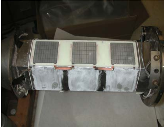
Figure 38. 200 W TEG for Hybrid Electric Vehicle Underassembly
