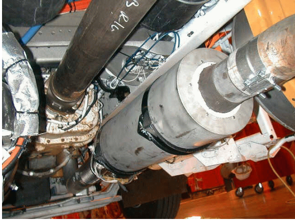
Figure 9. TEG Mounted on the Truck, View From the Bottom
