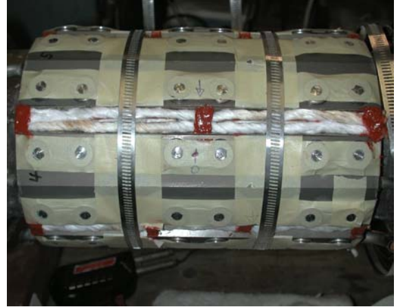
Figure 39. 200 W TEG. All modules are in place
