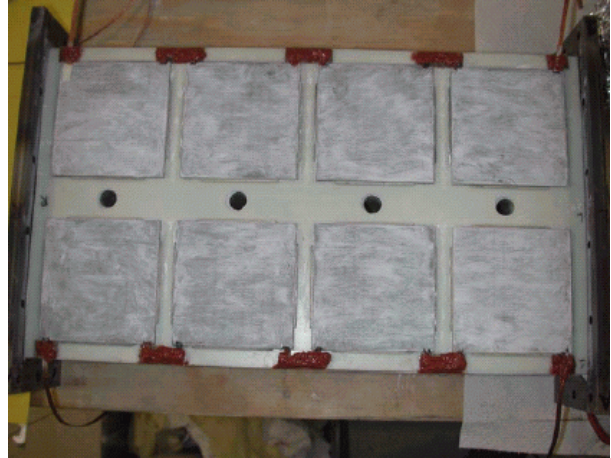
Figure 29. Additional Insulation Installed
