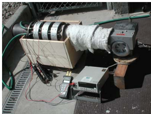
Figure 42. 200 W TEG Hot Air Blower Test
