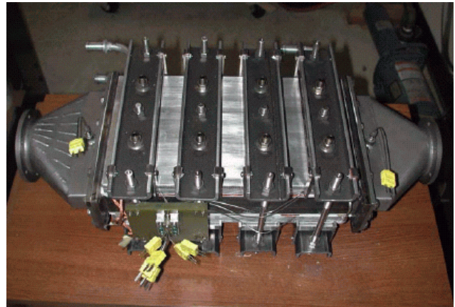
Figure 31. Assembled AETEG Without Case
