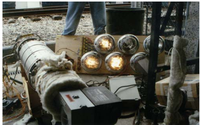
Figure 4. 1 kW TEG Test with Hot Air Blower. Light bulb loading board for obtaining matched load.
