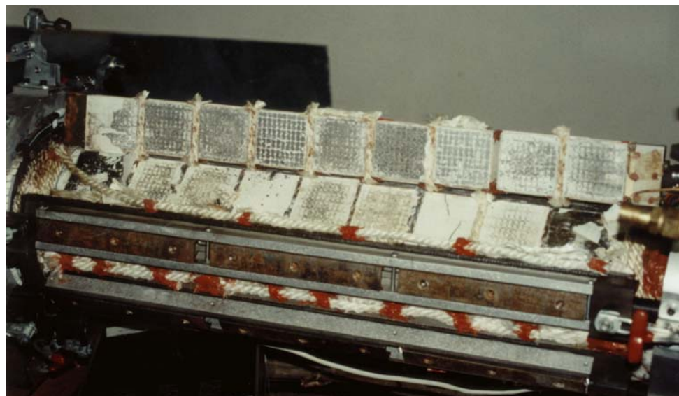
Figure 17 - Thermoelectric Array after Durability Test. All the modules, ceramic wafers, soft insulation, RTV in place.
