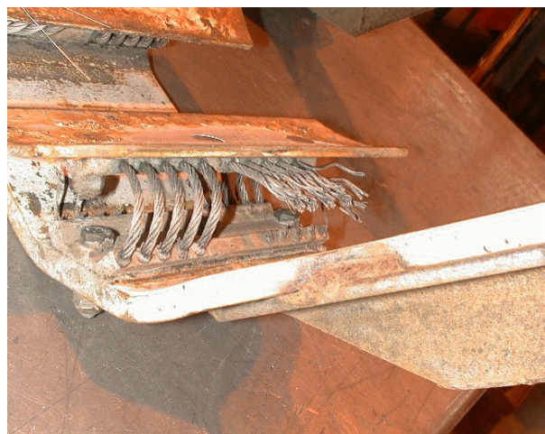
Figure 20. Shock Absorption System After Test
