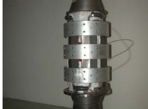
Figure 41. 200 W TEG Ready for Test
