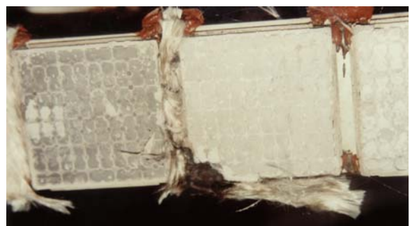
Figure 16. Thermoelectric Module #3 from the Array #4 Damaged by Thermocouple Electrical Short
