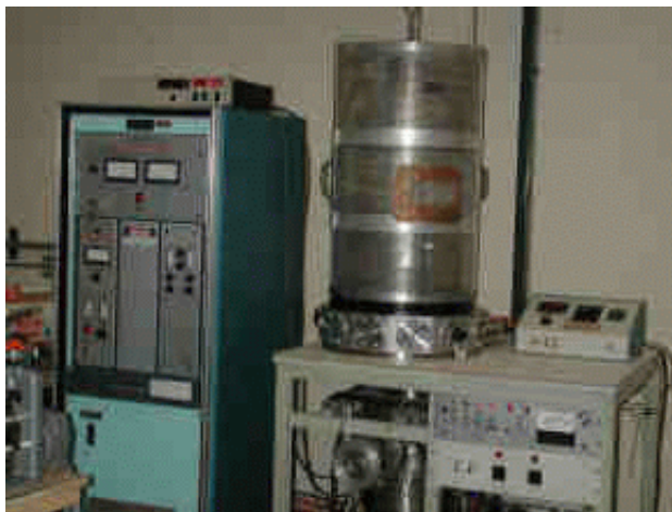
Figure 25. Overall View of Electron-Beam-Heated Deposition System
