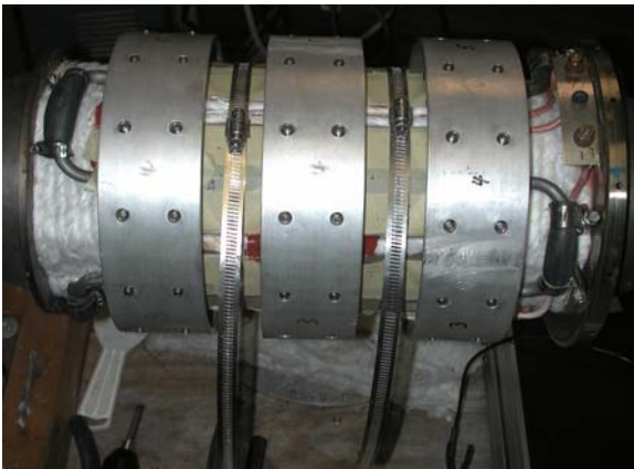
Figure 40. 200 W TEG Completely Assembled
