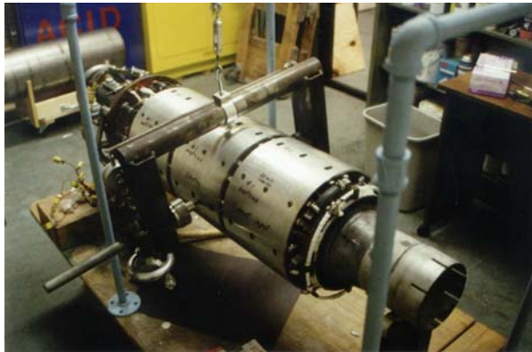
Figure 3. Applying Pressure to the Heat Sink
