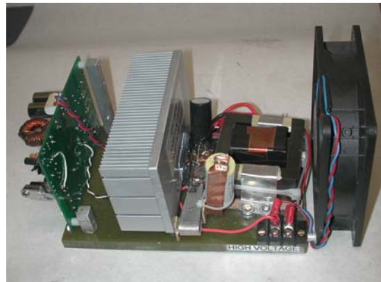
Figure 43. 200 W TEG Power Management System
