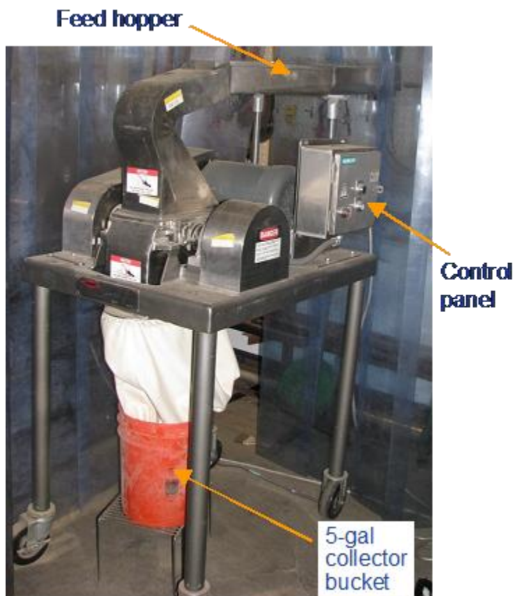
Figure 11. FitzMill installed in the test cell.
