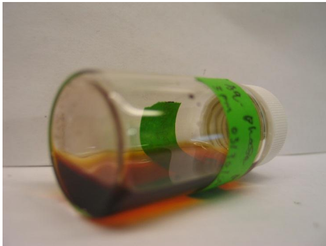
Figure 5.11 Hydrogenated WSBO at room temperature after heating treatment. Only a few of black oil droplets were created and separated from bulk solution.
