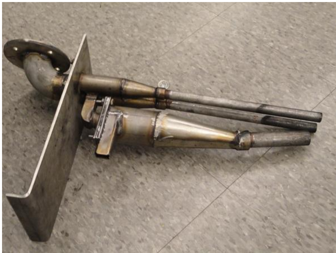
Figure 6.2 Two-stage cyclone consisting of a single cyclone followed by two smaller cyclones in parallel
