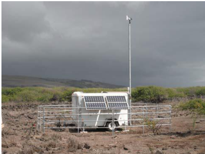
Figure 4.3 Solar powered, mobile SODAR with met-mast at Naalehu.
