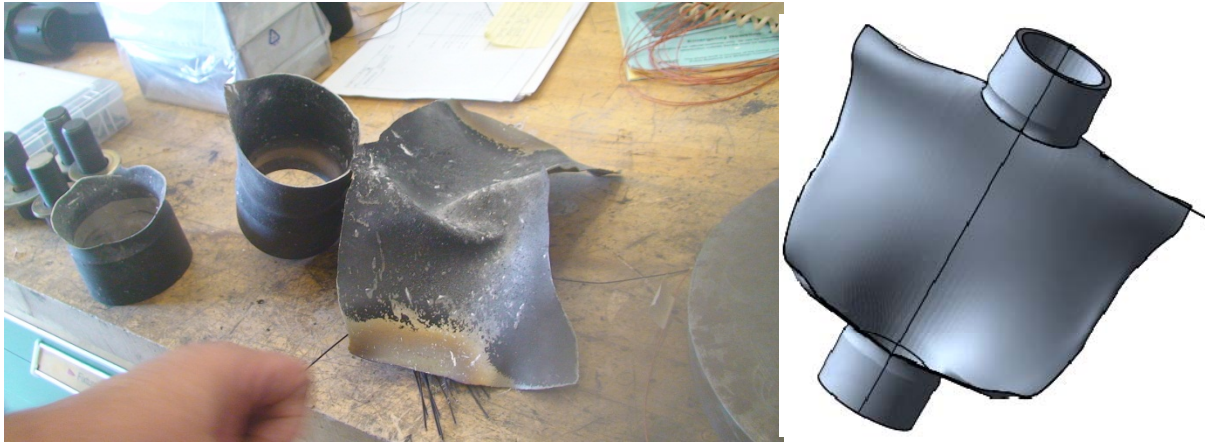
Figure 35. Comparison of experiment to simulation for deformed shape of the pipe-bomb after burst. Experiment on the left hand side, Analysis on the right hand side.
