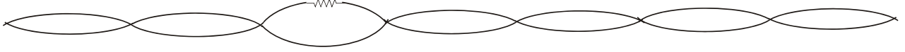
Figure 20. A twisted pair cable with a low impedance load in one wire.
