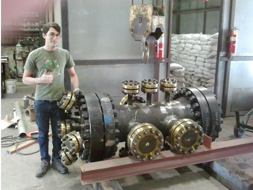
Figure 31. The high-pressure rubblized-bed reactor after pressure testing and certification, and prior to placement in the isolation room.
