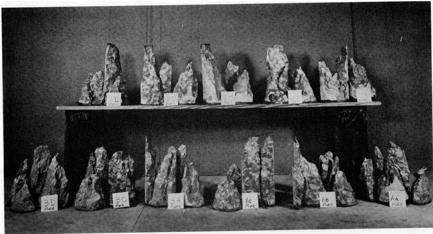
Six- by twelve-in. sections from cores 1, 2 and 3, taken from Prepakt bridge pier, after testing in compression at 90 days
