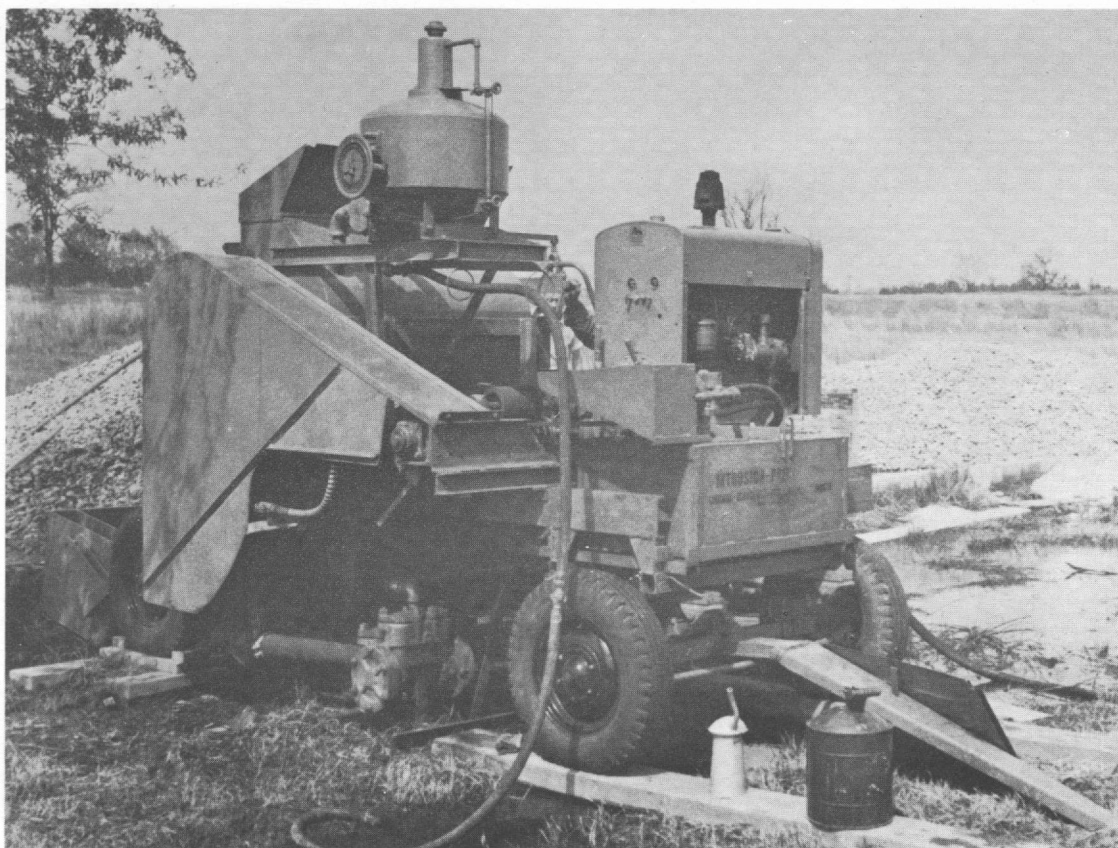
Figure 5. Grout mixing and pumping machine
