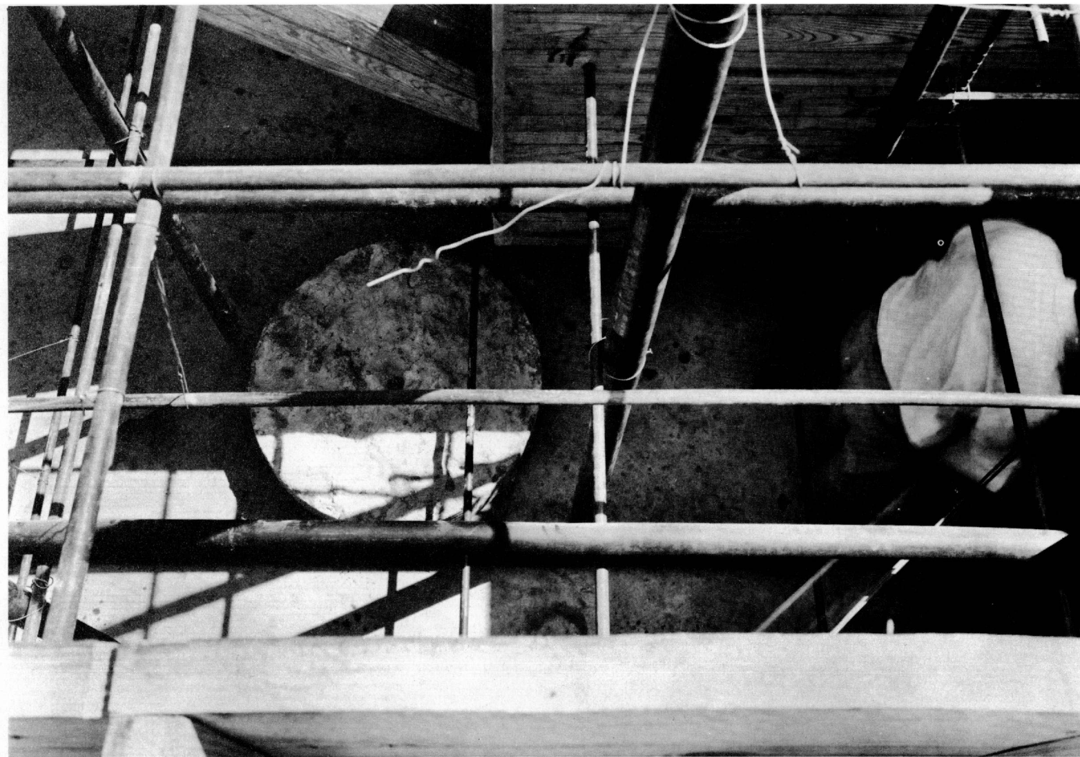
Sandblasted core in place on foundation of test block
