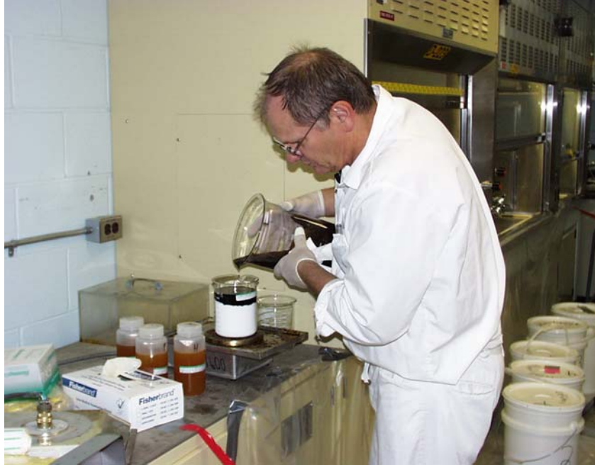
Fig. 1: Photograph Showing the Addition of Organic to Polymer
