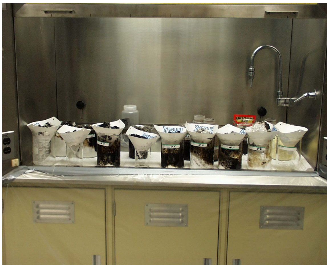
Fig. 3: Photograph of the Solidified Samples Being Tested for Free Liquid
