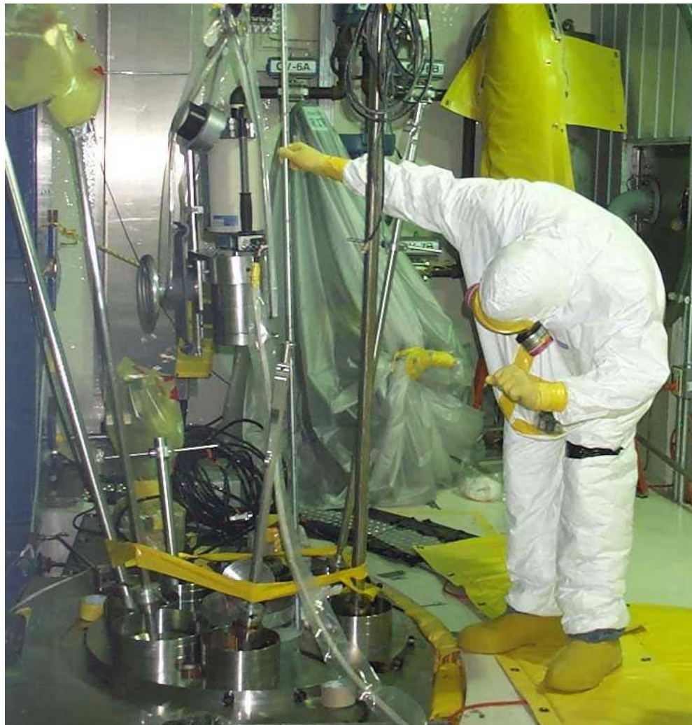
Fig. 3. Photo of HPGe detector suspended above the maintenance shield portal.
