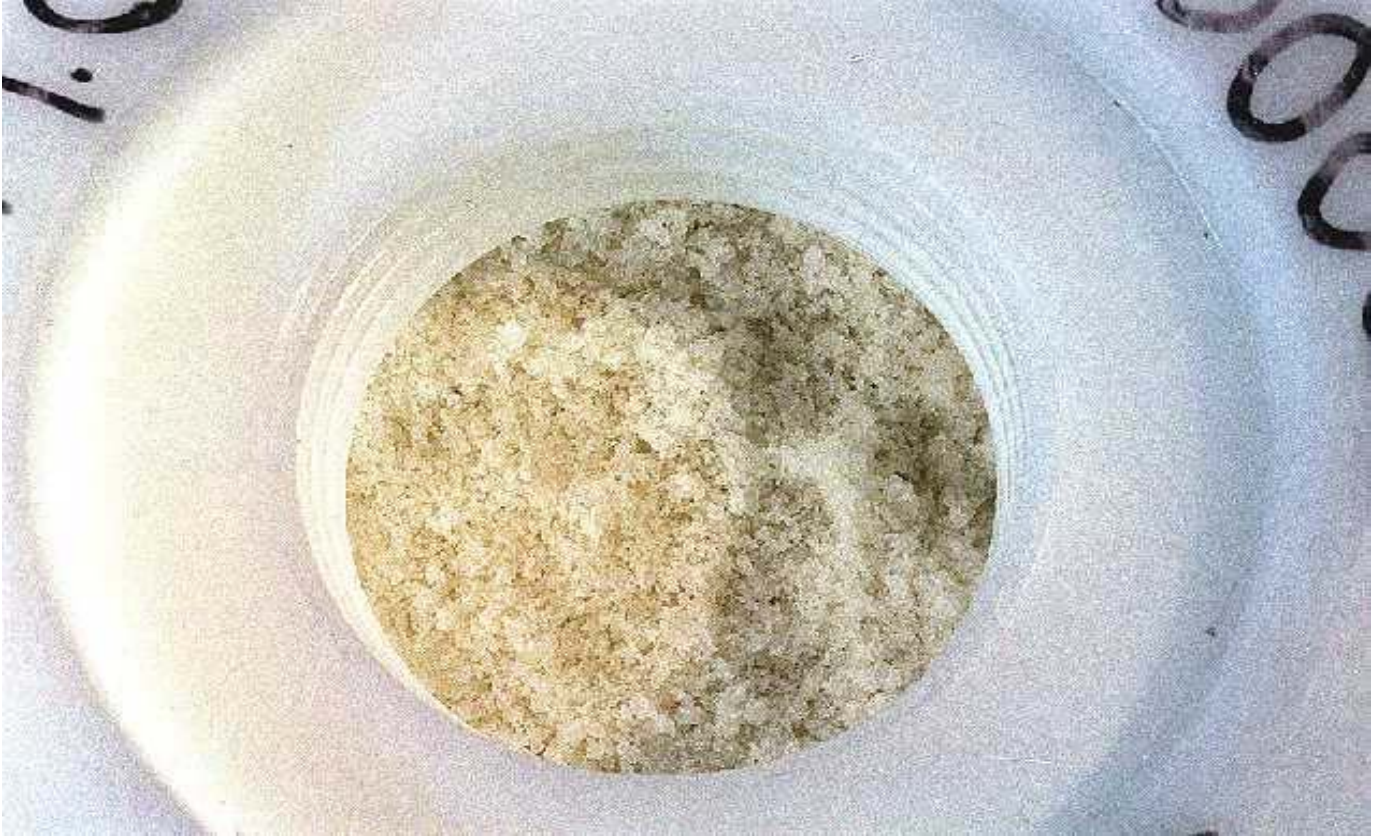
Fig. 1. Solidified Oil in a high density poly burial Liner- Top View
