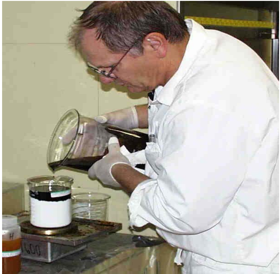
Fig. 3. HB-40 reactor coolant being solidified at Whiteshell Labs.
