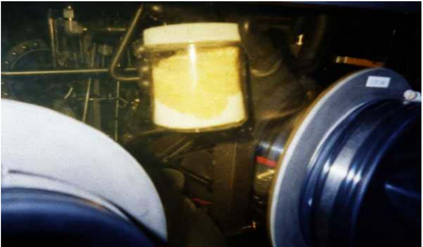
Fig. 2. High activity tritiated oil sample solidified inside a glovebox at Mound DOE Site.
