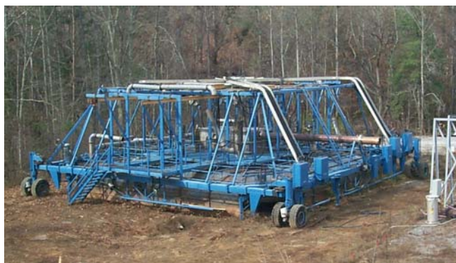
Fig. 4. In-situ Vitrification Hood System Structure.
