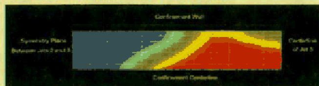
Figure 3. Contours of measured axial velocity 0.0279 m downstream from confinement inlet, illustrating the cross-stream resolution of scans in the measurement space.
