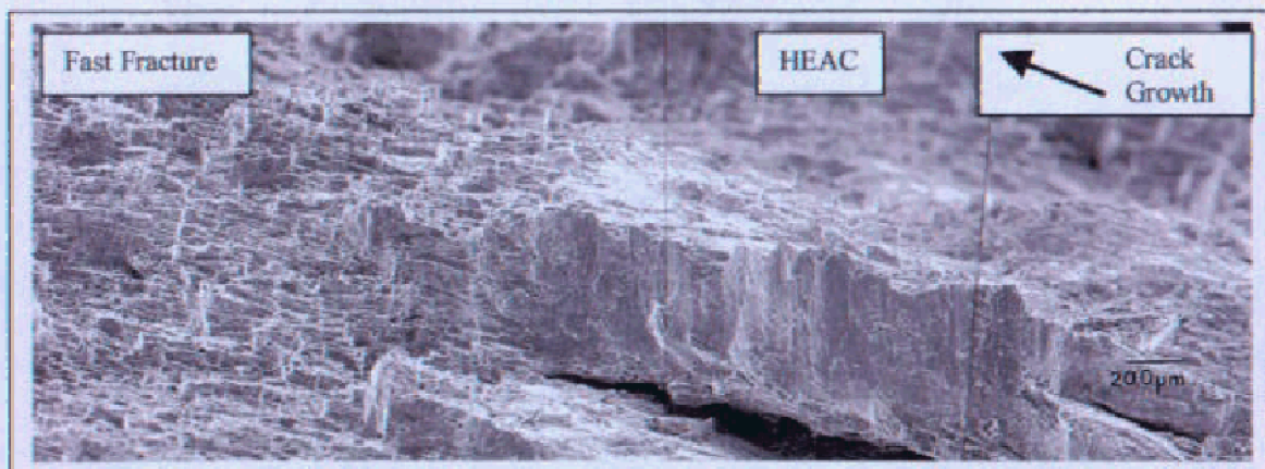
Figure 9. Scanning electron micrographs of the HEAC/Fast Fracture transition in low copper-OA tested in 60 °C, 90% RH air.
