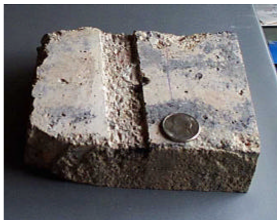
Figure 2: Laser ablation track in high density concrete. The track is twenty mm wide by 3 mm deep, and results from twenty passes of the laser, each ablating a 1 mm wide groove.
