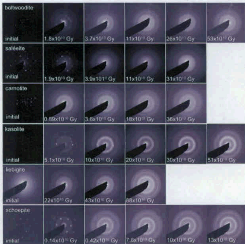
Fig. 2. The SAEDs of transition in the uranyl-phases as a function of the cumulative ionizing dose.
