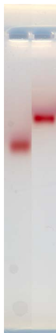
Figure 2.17: Spliced image of a single 10 cm agarose gel showing the migration of 5 nm gold compared to 10 nm gold coated with phosphine ligand.
