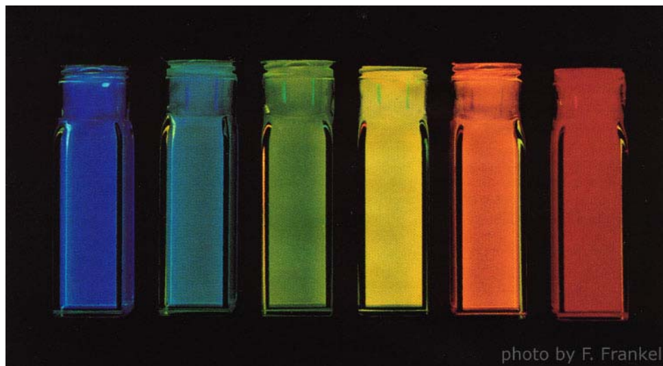
Figure 1.1: This figure from Dabbousi, et. al. shows a selection of six different sizes of CdSe/ZnS core/shell nanocrystals under excitation with a 365 nm source luminescing in a range of wavelengths between 470 and 620 nm, left to right.[4]
