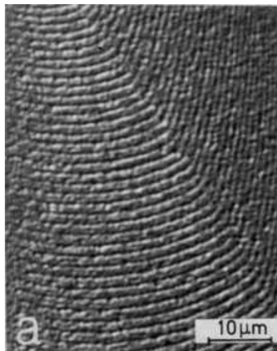
Figure 2.4: Scanning electron microscope image of the spiral growth steps around a screw dislocation nucleus, highlighted by Ge epitaxy. After [10].
