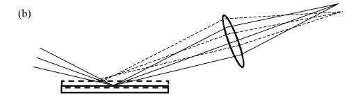
**Fig. 2.** Diagram illustrating optical response to (a) tilt of the target and (b) height change of the target. Angles and distances are greatly exaggerated compared to actual design for illustrative purposes.
