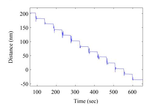
**Fig. 4.** Wafer height sensor measurement results from the implemented system operating in vacuum. The operating pressure was approximately  $9 \times 10^{-8}$  Torr. The wafer stage was actuated to generate a series of nominally 19-nm steps in height. The apparent jitter is believed to be real and attributable to poor damping of the wafer stage.
