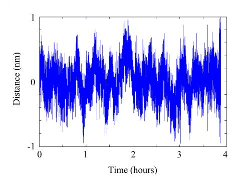
**Fig. 6.** Detail of the last few hours from the plot in Fig. 5. The plot demonstrates an rms noise floor of 0.26 nm (1.95 nm peak-to-valley).
