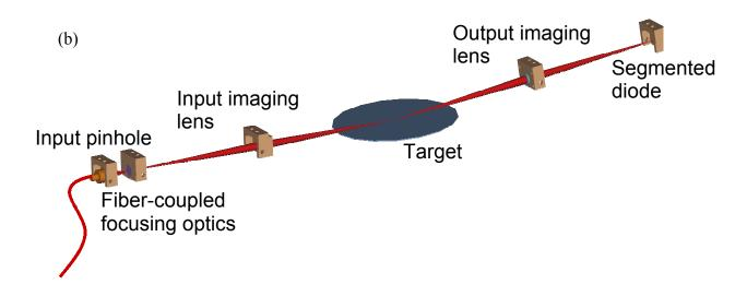
**Fig. 1.** (a) CODE V view of typical optical layout and (b) CAD rendering of system including fiber-optic source components.
