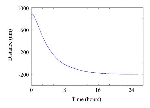
**Fig. 5.** Overnight plot of the height-sensor readings. A large height change (approximately 1  $\mu$ m) is seen over the first several hours and then the system stabilizes. This height change is real and is attributable to a thermo-electrically cooled CCD camera buried within the wafer stage being turned off at the end of the day.
