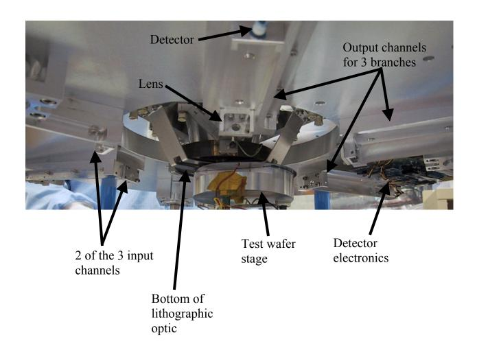
Fig. 3. Photograph of implemented wafer height sensor in testing fixture.
