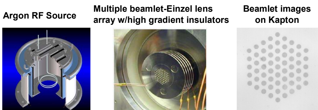
Figure 1: Results on the 100 kV Source Test Stand (STS-100): Sixty-one beamlets extracted from an RF-argon plasma source, through a grid supported by three multi-layer high gradient insulator stacks (not visible), with brightness and uniformity meeting requirements for heavy ion fusion.
