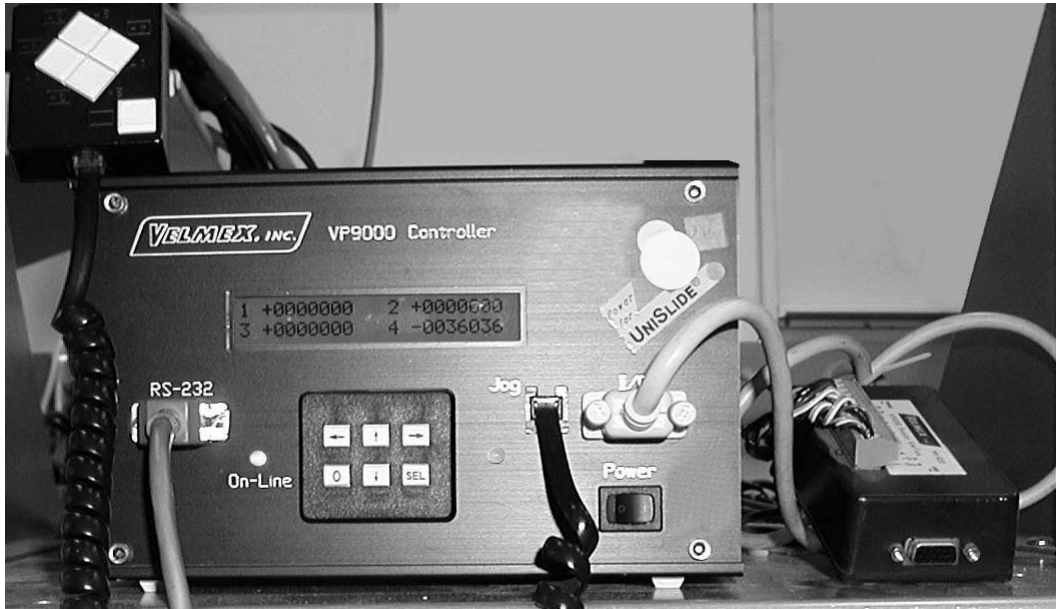
Figure 2-9. Picture of Velmex VP9000 stepper motor controller.
