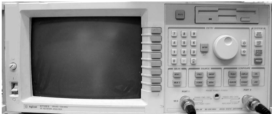
Figure 2-10. Agilent network analyzer used for spectral characterization.
