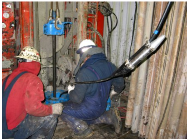
Figure A-10. Deploying VSP Array into Well
