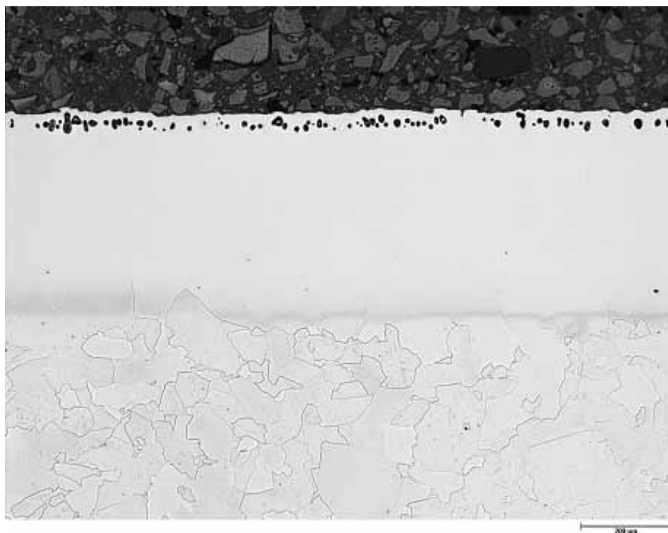
Figure 16: Optical Micrograph of the Grade 92 Chromized Sample (750°C)
