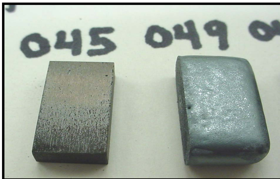
Figure 1. Condition of Alloy 188 (Specimen 045) and T-11 (Specimen 049) at the Conclusion of Trial #2
