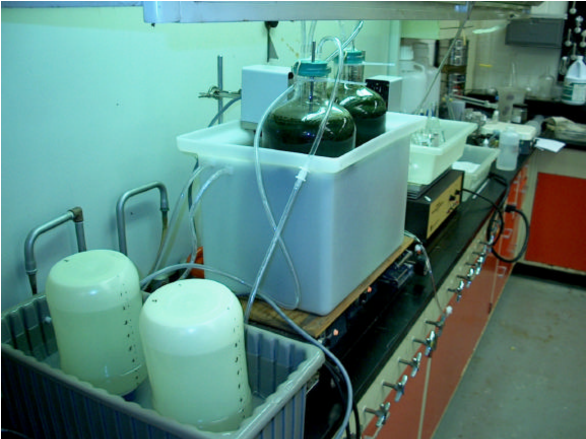
Figure 10. Gas Collection from Anaerobic Digesters
