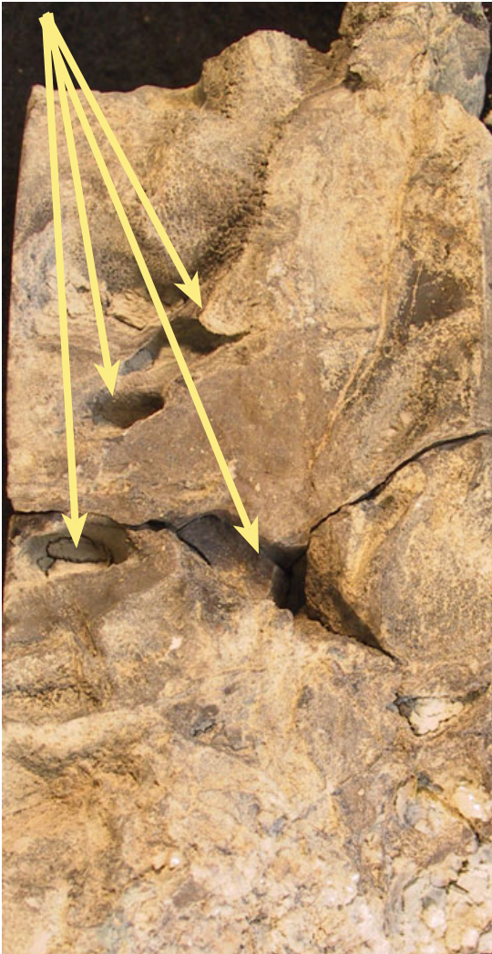
Figure 14. Core slab photograph of the side of a macrovug showing a solution-etched surface.
