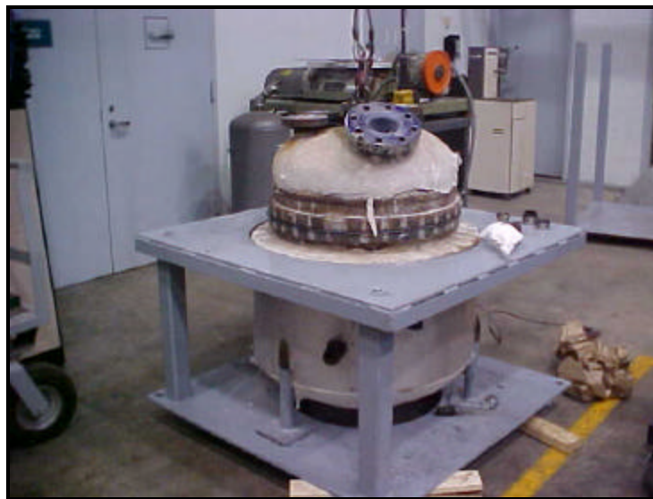
Figure 8. A Ceramic-lined Continuously Stirred Tank Reactor (CSTR) was fitted to new mounting structure and stand.
