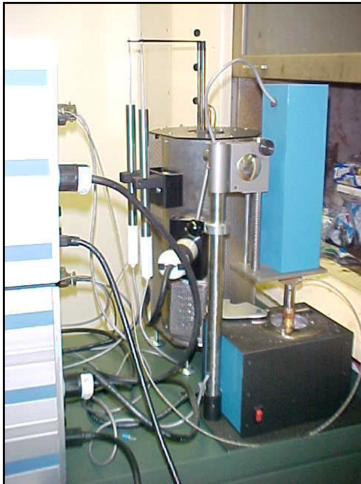
Figure 32. Dilatometer used for coal swelling trials.
