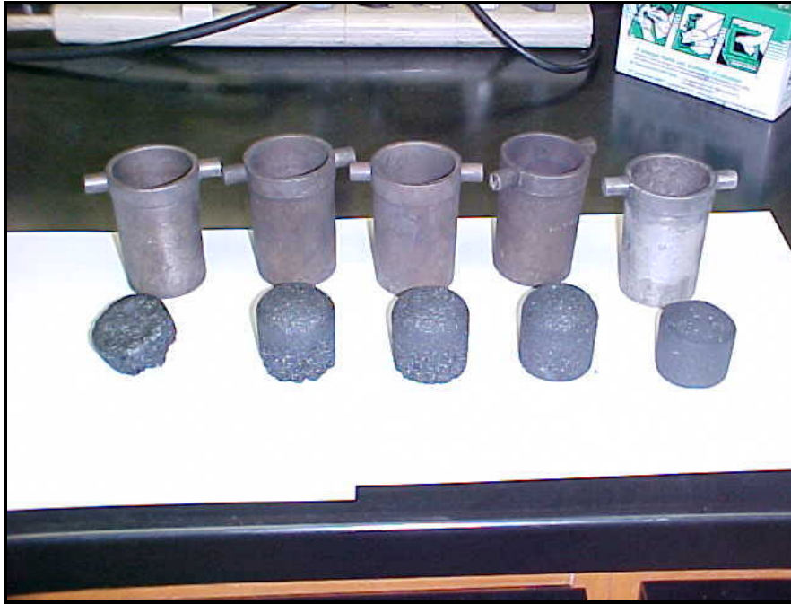
Figure 30. Carbon Foam Samples. The figure of merit was increased from left to right, corresponding with improved mechanical integrity. The sample on the left is the weakest and in fact crumbled in the test crucible.
