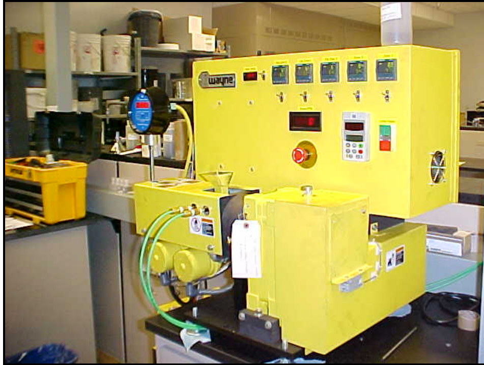
Figure 42. A Wayne fiber spinner and take-up reel were used to spin fiber from coal-derived pitches.
