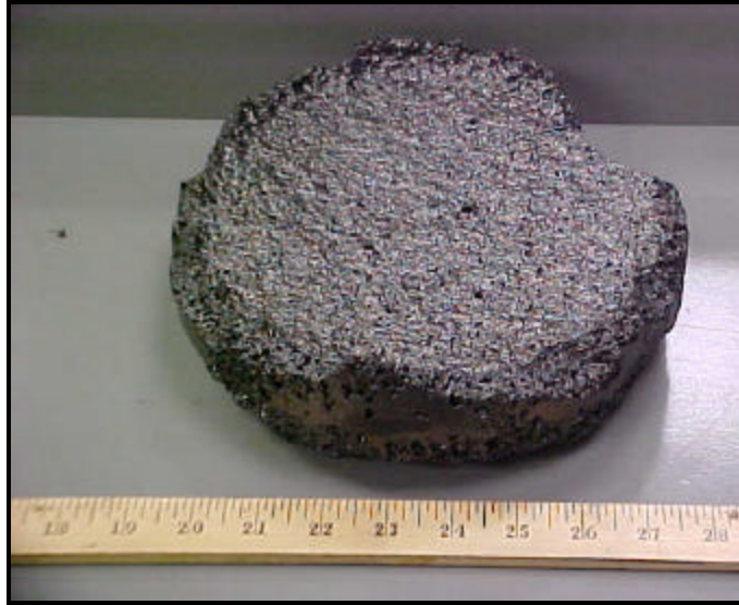
Figure 27. 8 inch diameter Synpitch-Derived Foam sample.
