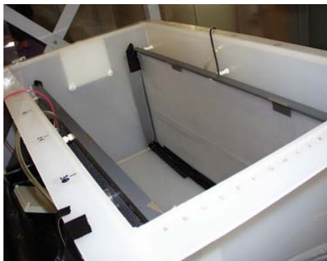
Figure 9 - Inside of EKAR cell showing soil barriers.
