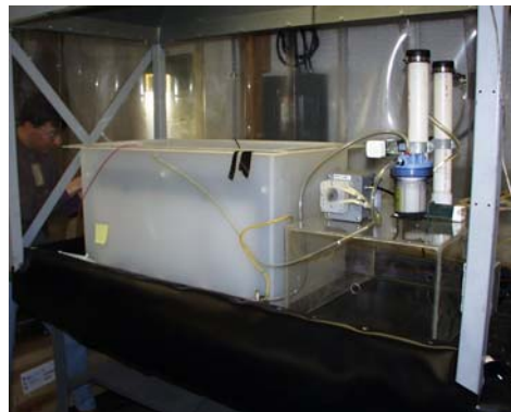
Figure 10 - EKAR cell. Pump, filter, and ion exchange columns are at right.
