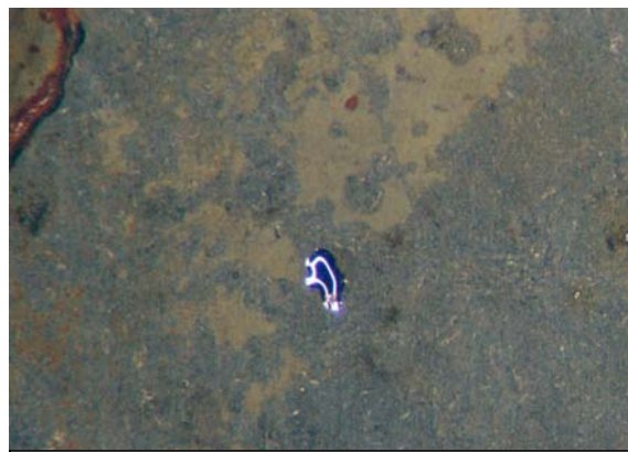
Figure 11 Elemental mercury droplet on the surface of the ECRTs cathode.
