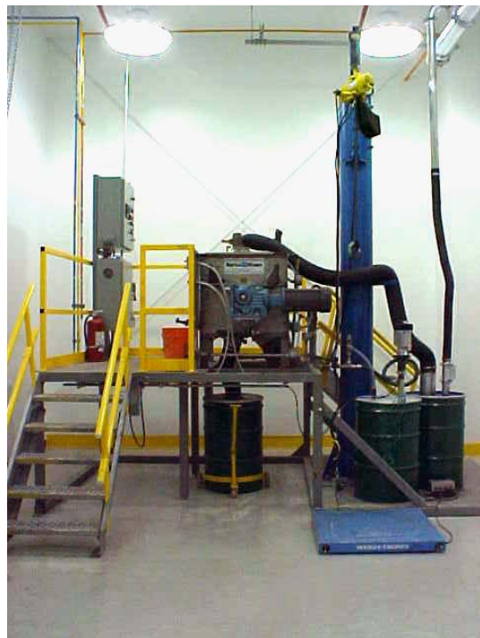
Figure 1 Stabilization skid designed and built for mercury contaminated soils.
