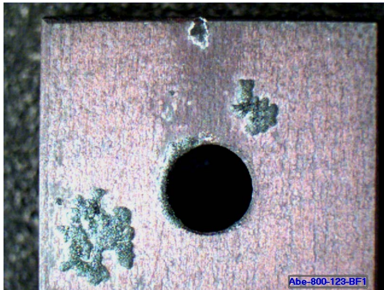
Figure 3. Oxide Nodules Formed on MARB2 (Abe) After 4,000 Hours of Exposure in 800°C Steam
