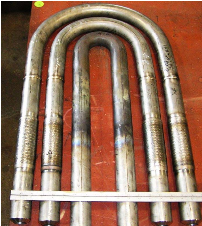
Figure 1 Demonstration Article "A" (nested USC superheater loops) during fabrication. Cast 50Cr-50Ni attachments will be welded to the assembly and all materials used in fabrication will be identified for display.
