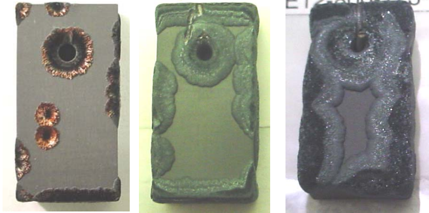
Figure 2. Growth of Oxide Nodules on SAVE12 in 800°C Steam (different specimens are shown)
