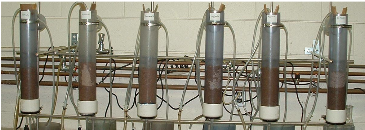
Figure 2: Percolation test columns assembled at MTU using equipment provided by Phelps Dodge Inc. Agglomerated ore is added to the column, and raffinate is circulated through the agglomerates continuously. The “slump”, or decrease in height of the ore, is also measured. The columns shown each contain agglomerates made with a different binder, and were initially all filled with the same amount of ore.
