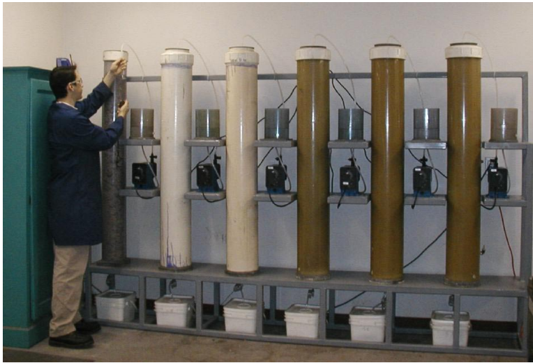
Figure 3: Leaching columns provided by Phelps Dodge set up for leach testing at Michigan Technological University. These columns are used for long-term testing for periods of several months, and provide the closest simulation of actual industrial heap-leaching behavior that can be achieved in the laboratory.
