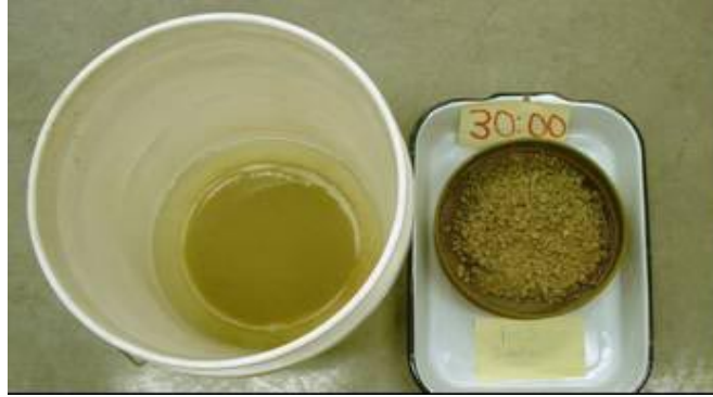
Figure 1: On the right is the 10 mesh screen holding the previously immersed agglomerates. The bucket on the left contains the fines which have been released due to the breakdown of the agglomerates.
