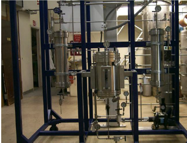
Figure 4. 4L-system for rapid aerogel production process optimization.
