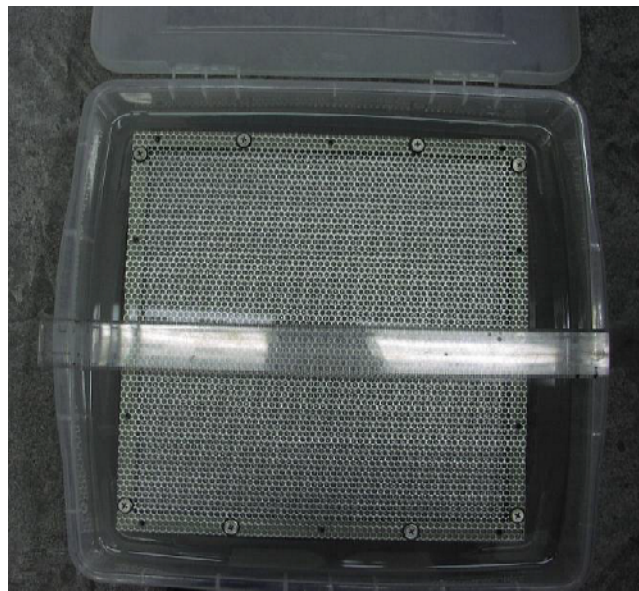
Figure 35. Aging of a 12"x 12" x 0.5" transparent aerogel in new mold.
