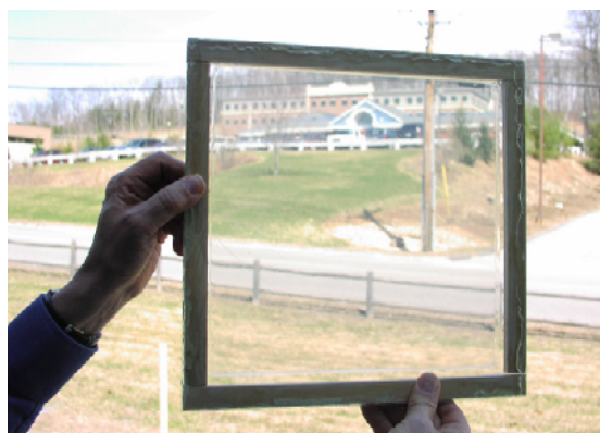
Figure 42. Hydrophobic and transparent POE/silica aerogel panel (1x1 ft) made using Mn 4000.
