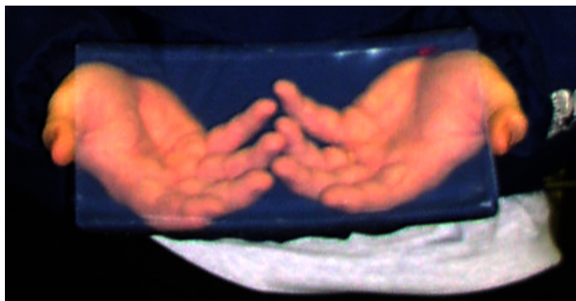
Figure 40. Panel of Ormosil POE/SiO 2 aerogel under flexural stresses.
