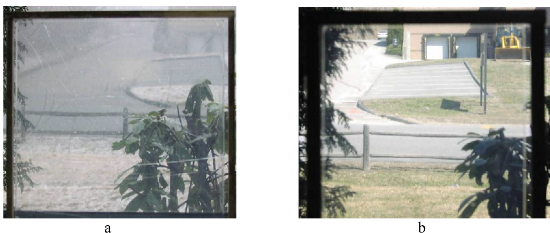
Figure 41. Transparent aerogel panels made during the last quarter: a) one of the first attempts which contained cracks and b) the most recent attempt is crack free.
