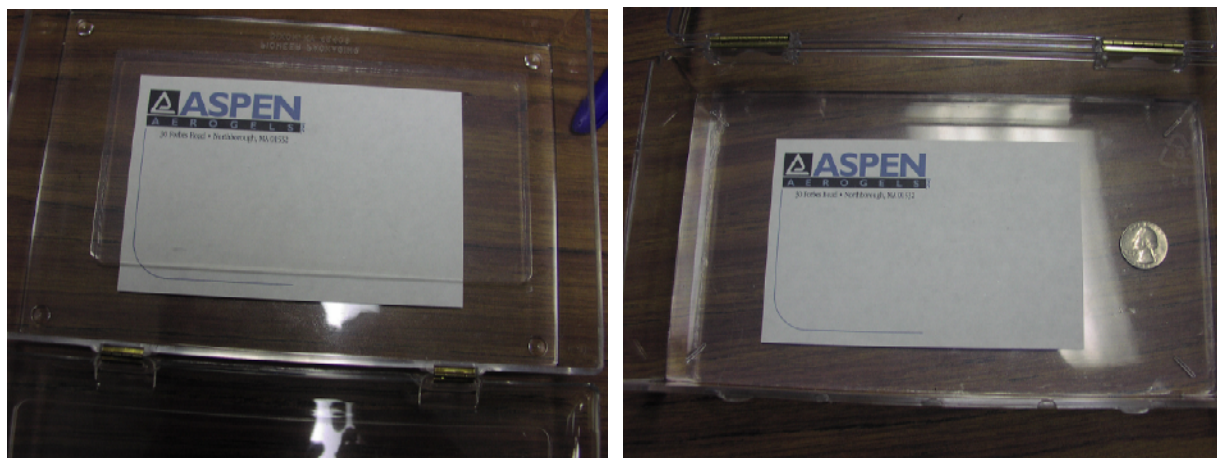
Figure 39. Large pieces of crack free Ormosil aerogel monolith with size of 10 x 20 x 1.1 cm (left) and with size of 15.5 x 26 x 1 cm (right).
