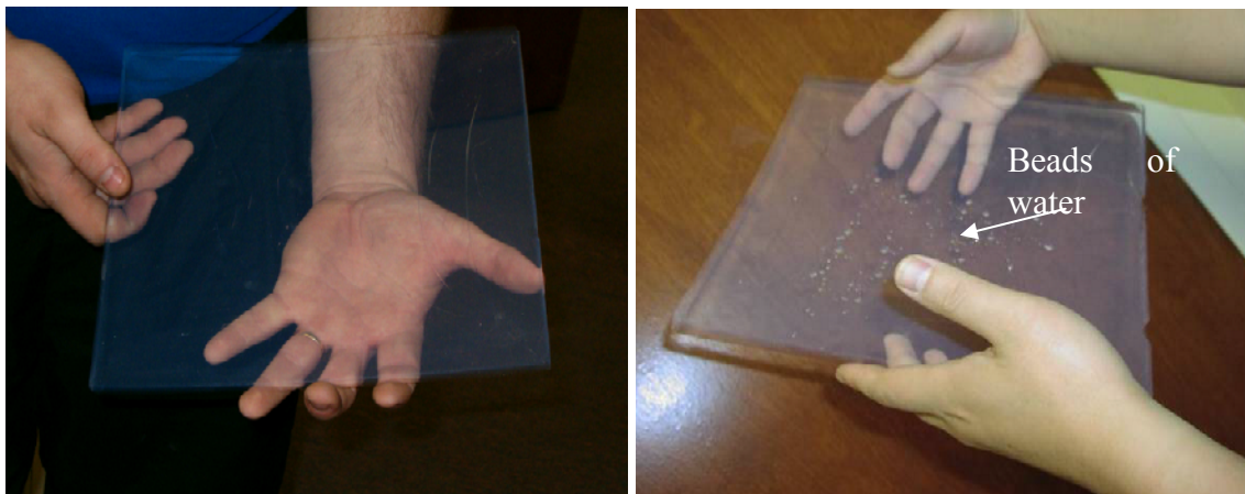
Figure 43. Hydrophobic and transparent POE/silica aerogel panels (1x1 ft) made using Mn 2000.
