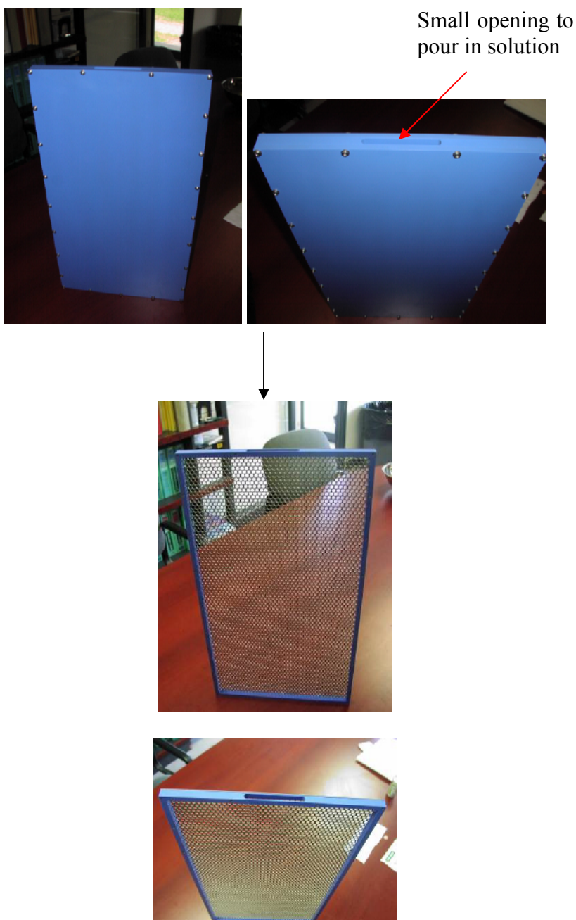
Figure 36. New 2'x 1' closed mold and perforated steel plates used to hold the gel.
