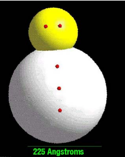
Figure 4. Representation showing the relationship between micropores (small red spheres), mesopores (yellow sphere—head) and macropore (white sphere—body).
