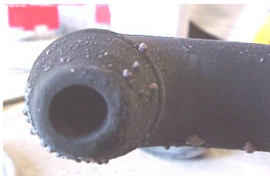
Figure 3.6 Tip of the Sampling Probe after Testing in the Pilot-scale Facility
