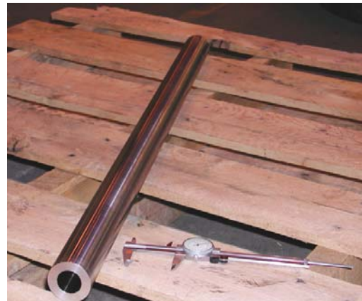
Figures 1 and 2 Images showing longitudinal sections machined from a SAVE12 pipe (left) and a tube machined from a SAVE12 section (right).
