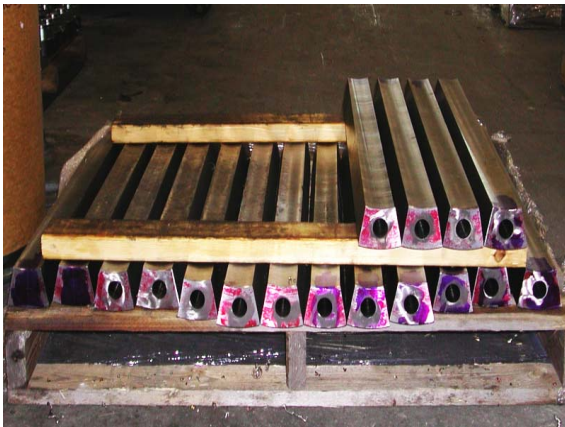
Figures 1 and 2 Images showing longitudinal sections machined from a SAVE12 pipe (left) and a tube machined from a SAVE12 section (right).
