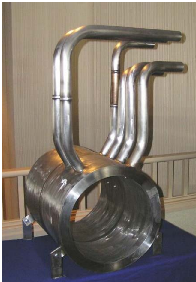
Figure 1. Image showing Alstom's mockup assembly that was built to demonstrate the progress that has been made while studying the fabricability of the CCA 617 and Super 304H materials.
