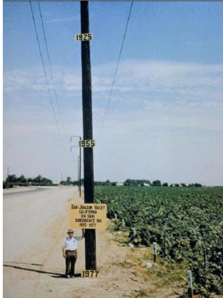
Figure 7. Land Subsidence in the San Joaquin Valley Southwest of Mendota Between 1925 and 1977
