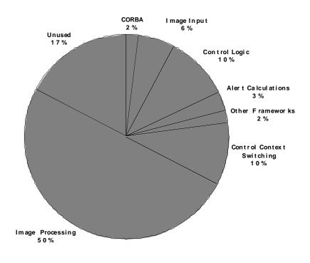
Automatic Alignment CPU Utilization per Processor
