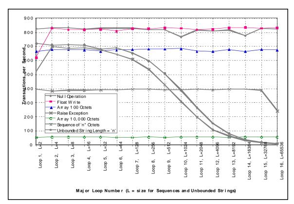
Figure 5 Comparative results of speed of various CORBA types
