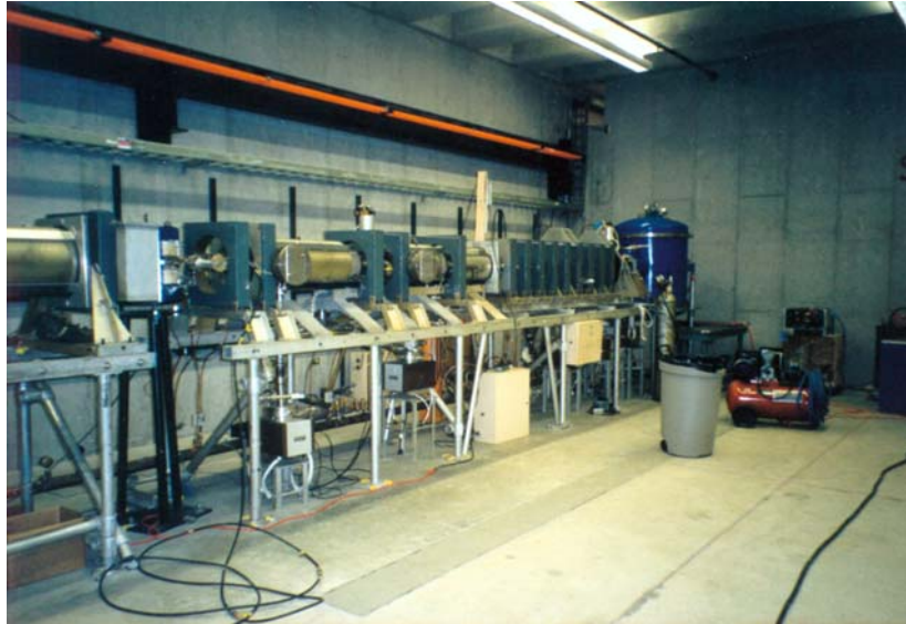
Figure 4. L-Band electron LINAC at the Idaho Accelerator Center.
