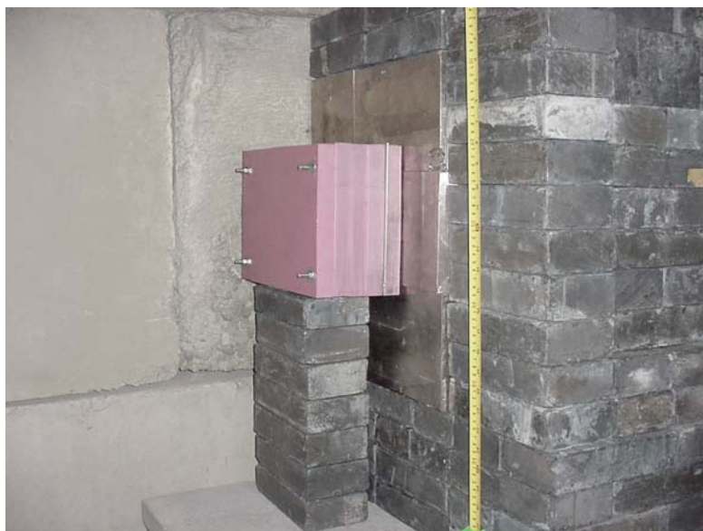
Figure 8. Downstream side of the completed neutron filtering assembly, with foil positioning shield in place.
