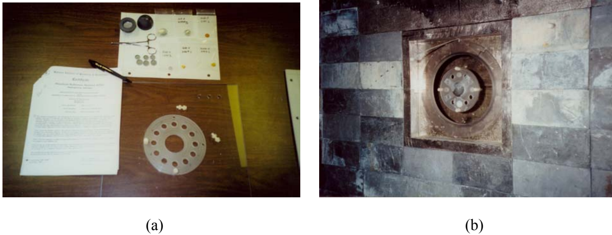
Figure 5. Activation foil plate (a) positioned in the WSU epithermal neutron beam source plane (b).
