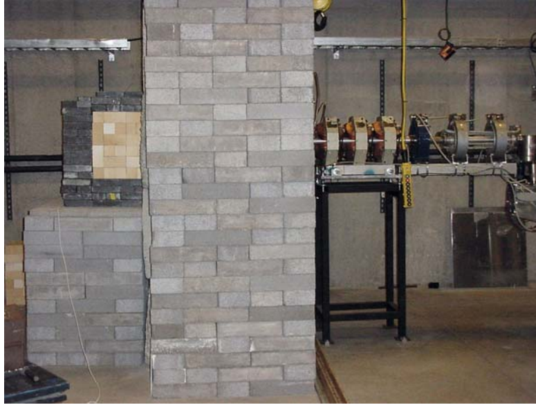
Figure 6. View perpendicular to the electron beam axis, showing the shielding wall, the accelerator drift tube on the right, and the filter/moderator/reflector assembly on the left.
