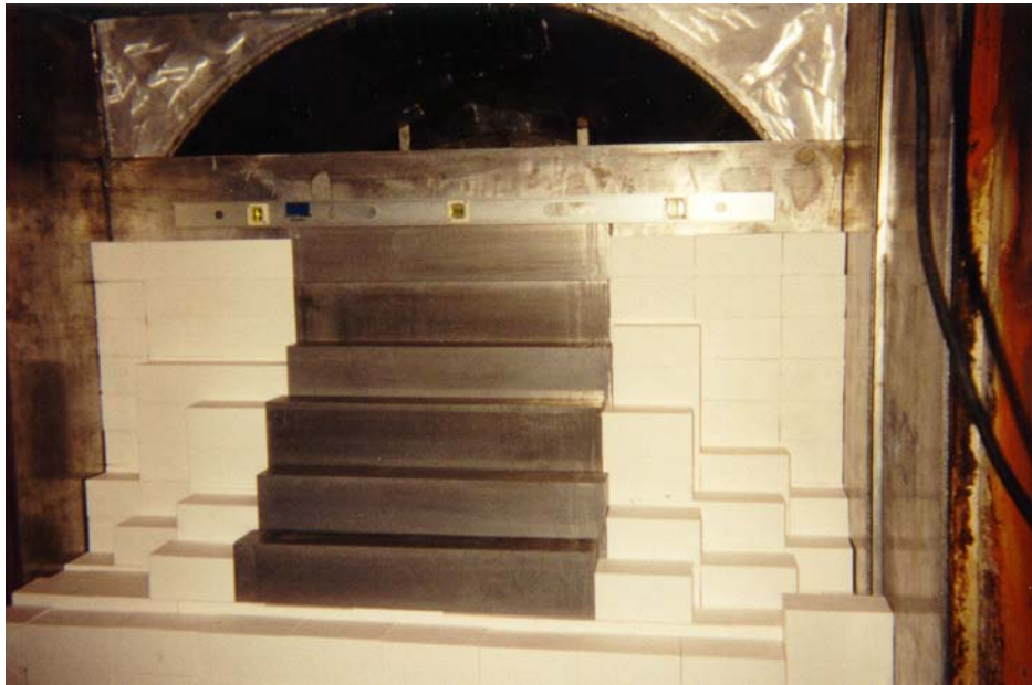
Figure 7. Partially completed WSU filter-moderator assembly, showing the FLUENTIAL and alumina blocks, and the boral backing sheet. Note the offsets in both directions.
