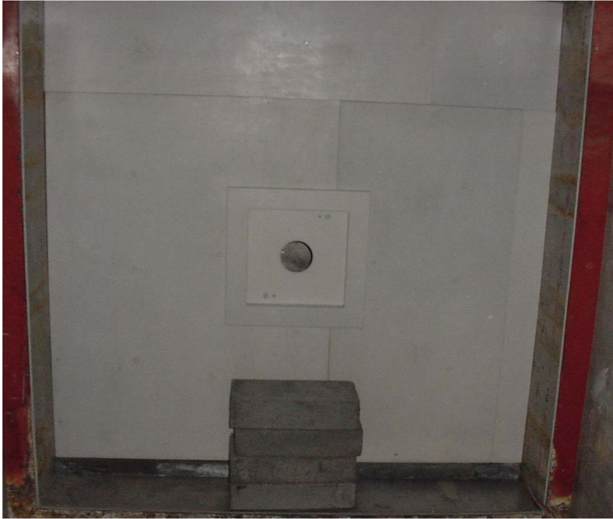
Figure 24. Outer face of the filter-moderator region showing lithiated polyethylene in place. The four inch collimator is in position.
