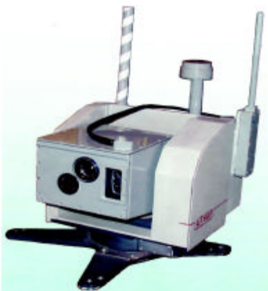
Figure 2. Russian Gamma Locating and Isotopic Identification Scan Head
