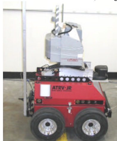
Figure 3. Combined Robotic platform and Russian Scan Head
