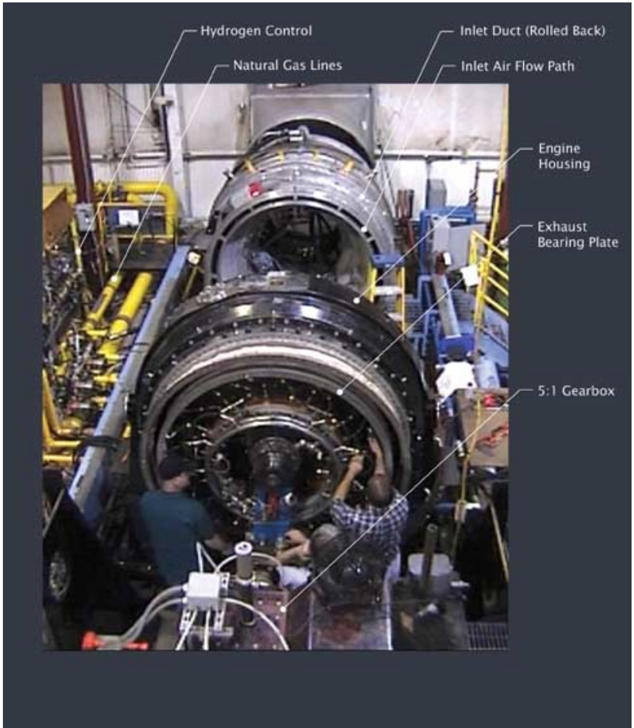
Engine Prepared for Assembly Figure 3.3
