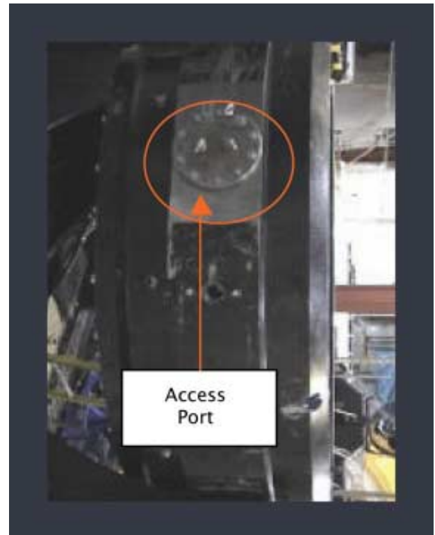
Combustor Access Port Figure 3.53
