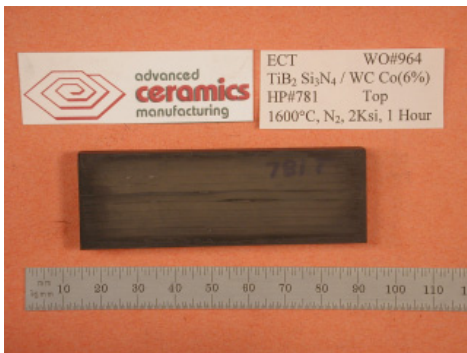
Figure C1K1 82.5% TiB 2 -(2.5%)Si 3 N 4 /17.5%WC-(3%)Co
