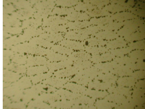
Figure D1A2 WCCo(6%) / WFeNi (693T) 50x
