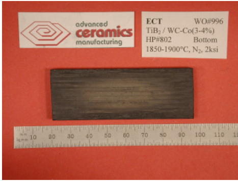
Figure C1P1 82.5% TiB 2 -Si 3 N 4 /17.5%WC-(3%)Co
