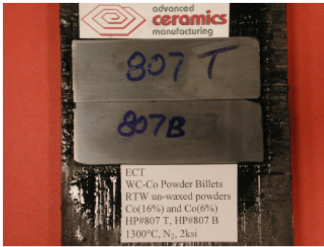
Figure D2F1 WC-(16%)Co powder billet top, WC-(16%)Co powder billet bottom
