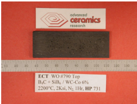
Figure B1H1 82.5\%B_4C -(6%) SiB_6 /17.5% WC -(6%) Co
