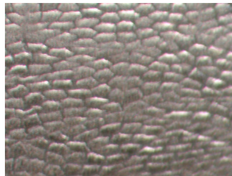
Figure C1N2 82.5% TiB 2 -(2.5%)Si 3 N 4 /17.5%WC-(6%)Co
