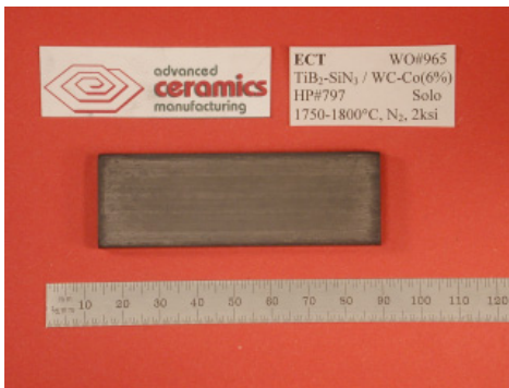
Figure C1N1 82.5% TiB 2 -(2.5%)Si 3 N 4 /17.5%WC-(6%)Co
