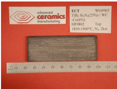
Figure C1O1 82.5% TiB 2 -(2.5%)Si 3 N 4 /17.5%WC-(6%)Co
