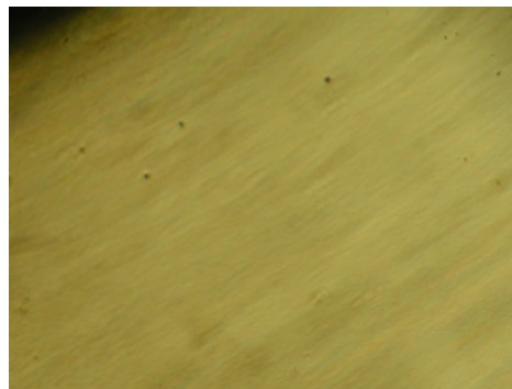
Figure D2H2 WC-(14%)Co powder billet
