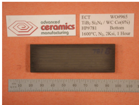
Figure C1L1 82.5% TiB 2 -(2.5%)Si 3 N 4 /17.5%WC-(6%)Co
