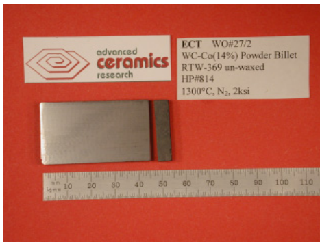
Figure D2H1 WC-(14%)Co powder billet
