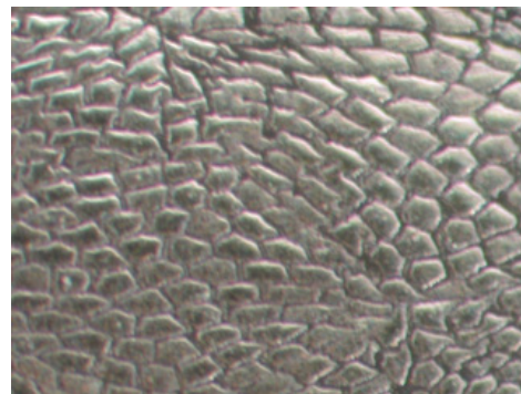
Figure C1O2 82.5% TiB 2 -(2.5%)Si 3 N 4 /17.5%WC-(6%)Co
