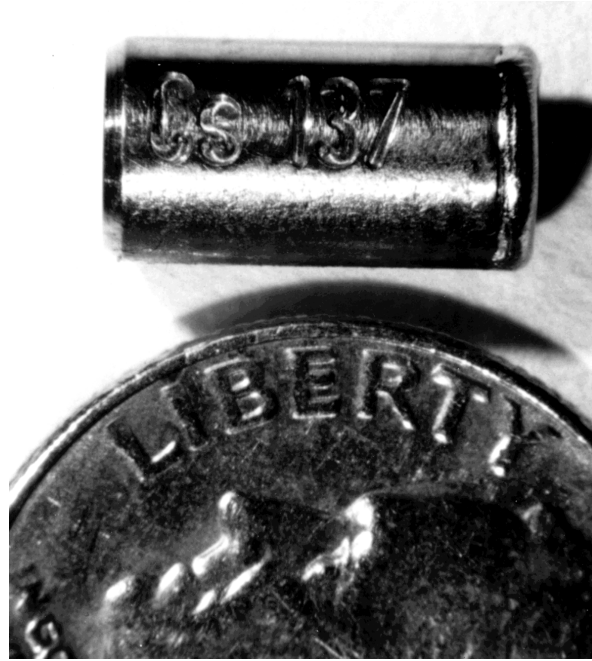
Figure 1. Pollucite capsule, shown with dime for scale.
