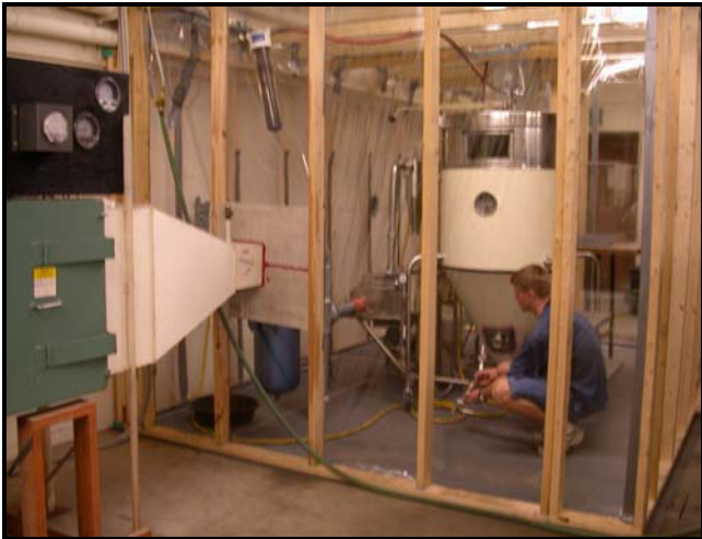
Figure 9. Photograph of the Spray Drying System Showing the Chamber and HEPA Filtration System.
