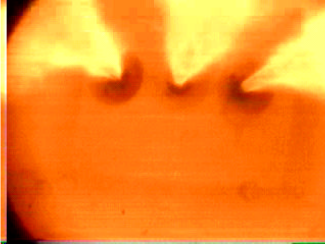
Figure 4.5. Flame images taken with all burners at full load, 1.5 MM Btu/hr.
