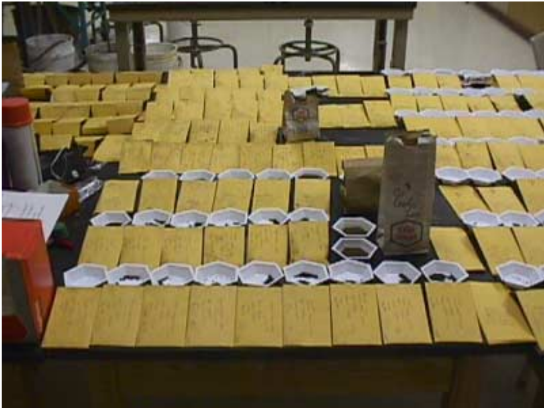
Figure 2: Iron ore samples divided into the different particle sizes after the iron assays and specific gravity was completed.
