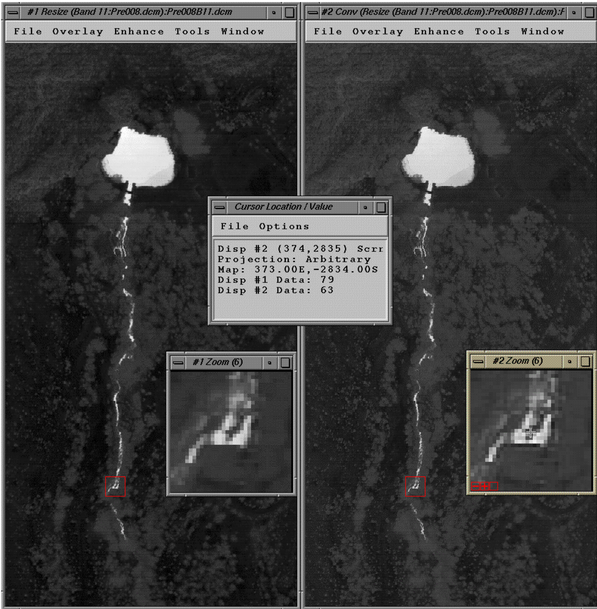
Figure 8. Behavior of the Wiener filter in the neighborhood of a small low-temperature anomaly.
