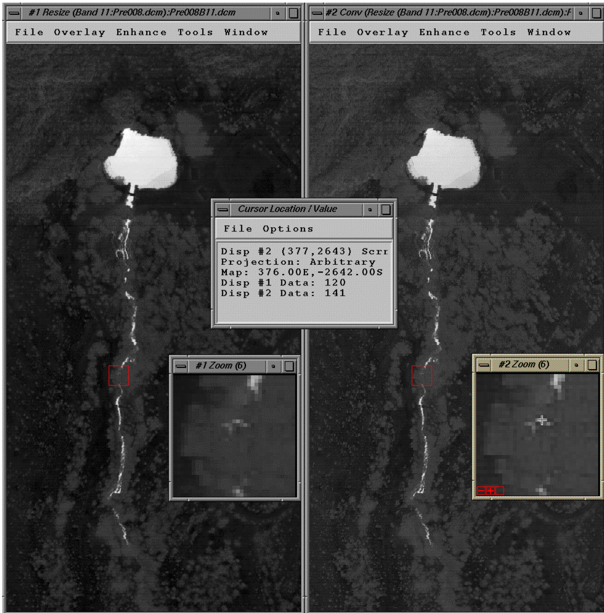
Figure 7. Behavior of the Wiener filter in the neighborhood of a small weak high-temperature anomaly.
