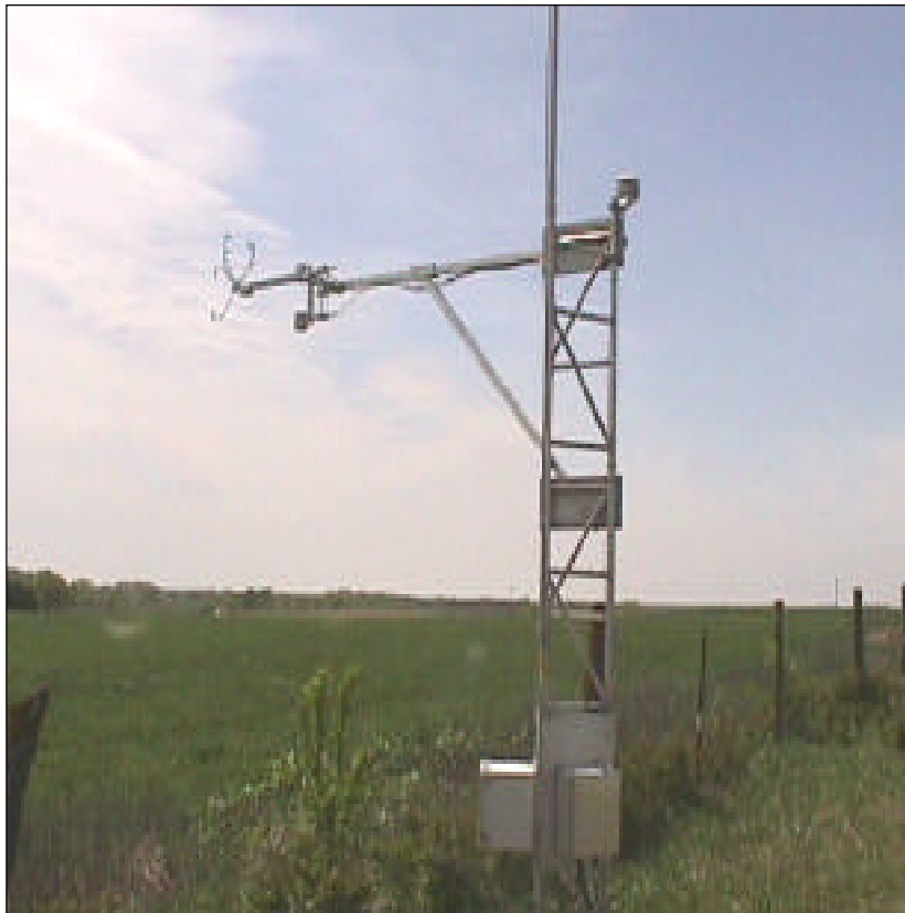
Figure 2. The ECOR system mounted in a field. The sonic anemometer is at the end of the boom on the left. The infrared hygrometer is to the right of the anemometer.
