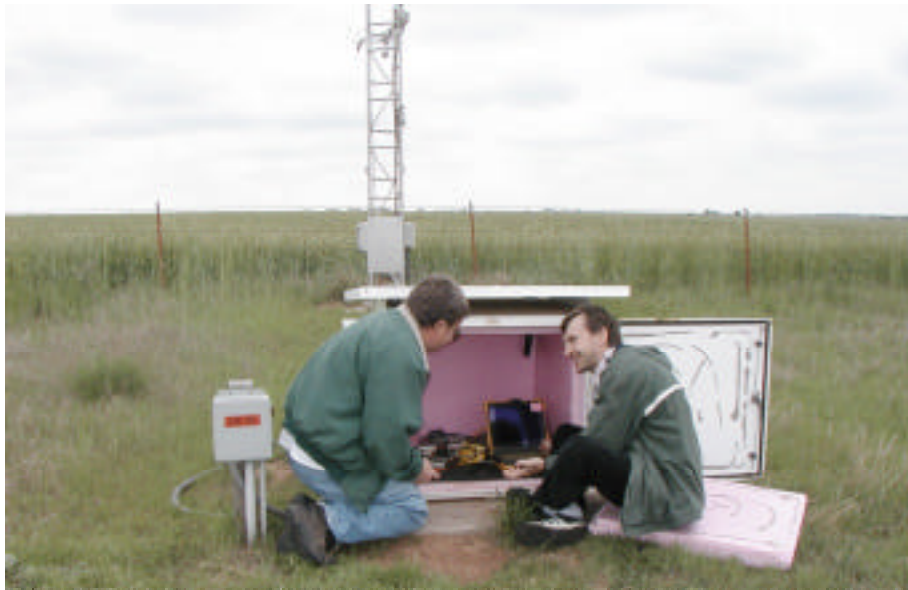
Figure 1. ARM field technician Mike Rainwater (left) and ECOR instrument mentor Dr. Mikhail S. Pekour install new computer equipment in the ECOR shelter.
