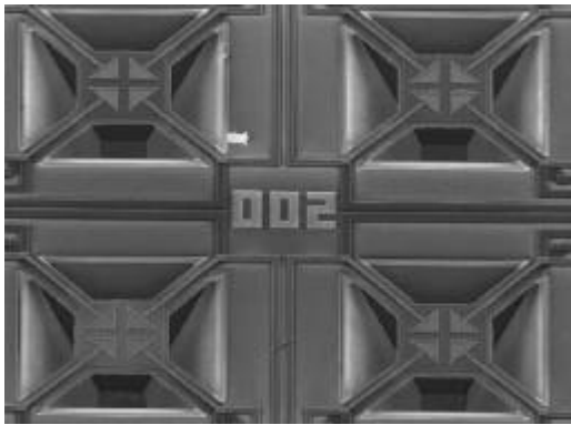
Figure 3. 4-element microhotplate array used to develop prototype gas
