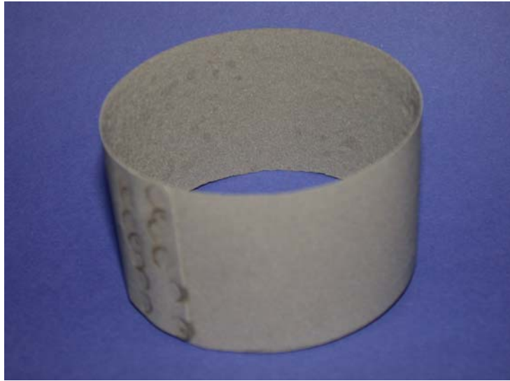
Figure 9. Resistance spot welded porous cylinder of sintered Ni-Cr-2xAl-Fe powder.
