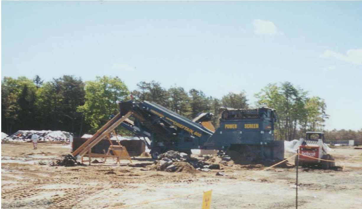
Figure 2. The half-inch vibratory screen unit (Powerscreen Chieftain 600)
