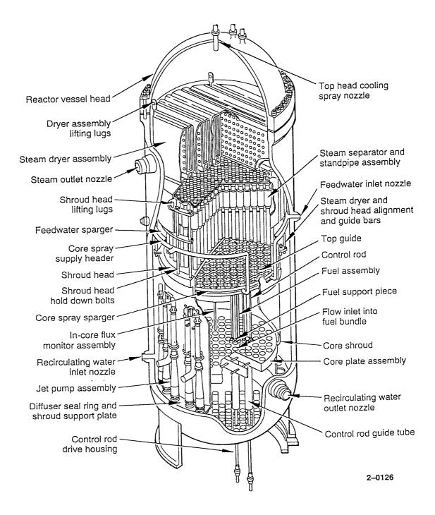
Fig. 1. BWR/3 or BWR/4 reactor vessel internals
