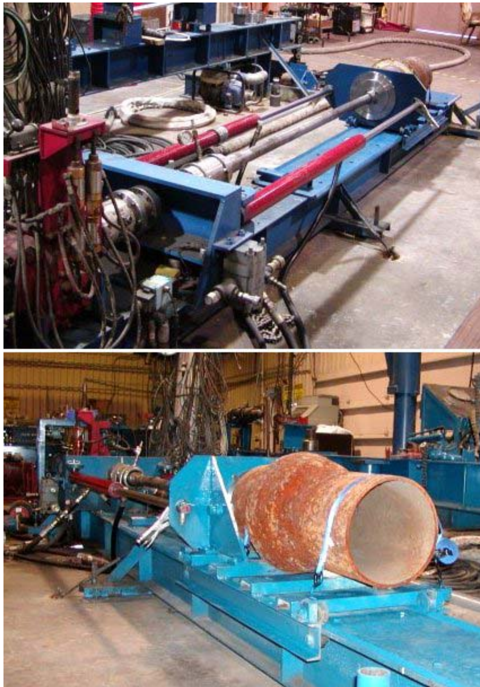
Figure 17. Fixture for Testing Joint-Cleaning Assembly
